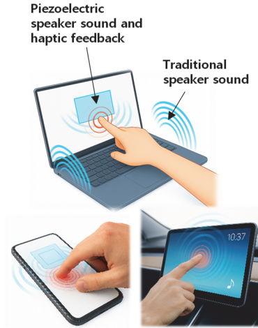
Fig. 6. Conceptual illustrations of display-integrated piezoelectric actuators enabling sound generation and haptic feedback. Thin piezoelectric speakers embedded in laptops, smartphones, and automotive display panels emit acoustic waves while simultaneously providing localized tactile vibration in response to user touch [14,32,36].
