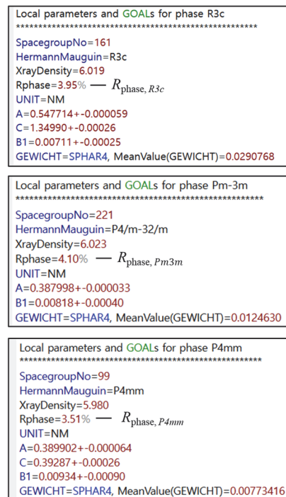
Fig. 20. Identification of problematic phases using R_{phase} values.
