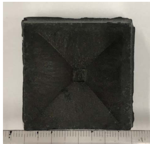
Fig. 3. YBa 2 Cu 3 O 7 superconducting bulk by top seeded melt growth.
