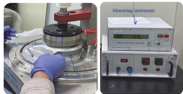
Fig. 9. Measuring tanδ of XLPE insulation.
