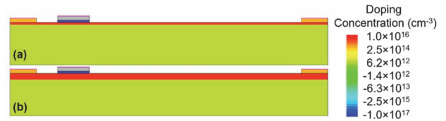
Fig. 2. NiO/ \text{Ga}_2\text{O}_3 heterojunction FET with epi thicknesses of (a) 100 nm and (b) 300 nm.
