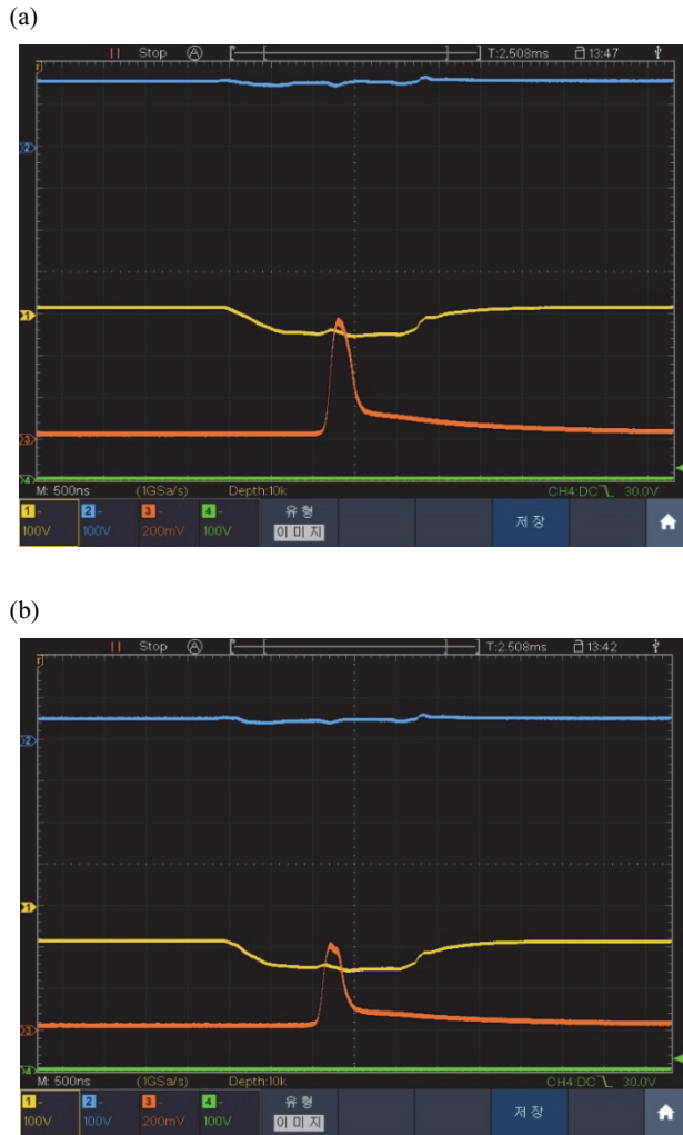
Fig. 3. Measured the write discharge characteristics when the scan and write pulses were applied during a write period in the conventional (a) and single sustain (b) driving methods.
