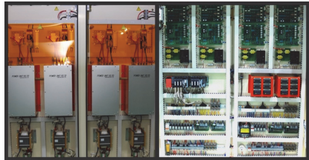
Fig. 2. Induction heating oscillator system.
