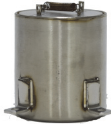
Fig. 3. Thermal battery applied by the synthesized heat powders.
