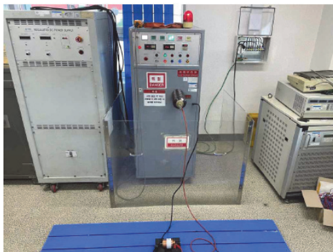
Fig. 11. AC withstand voltage test.
