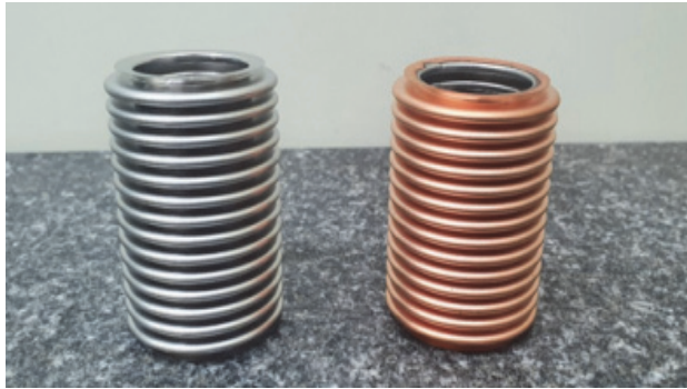
Fig. 4. VVC bellows (before and after Cu-plating).
