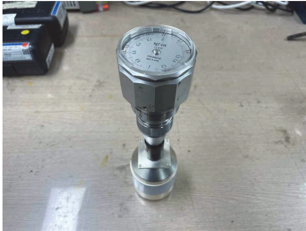
Fig. 13. Rotating torque test on movable part.
