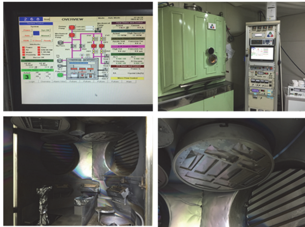
Fig. 3. E-beam deposition system.
