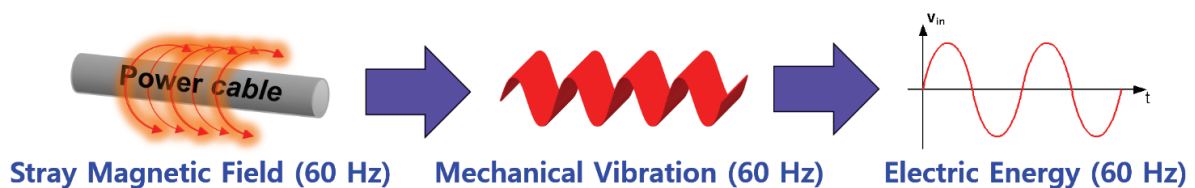
Fig. 1. The concept of magneto-mechano-electric conversion.
