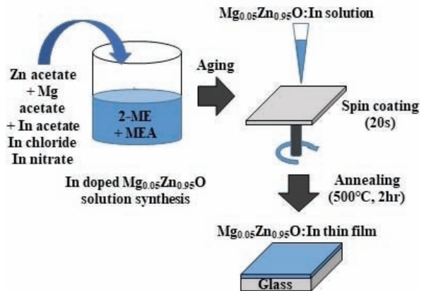
Fig. 1. Schematic diagram of the sol-gel method.
