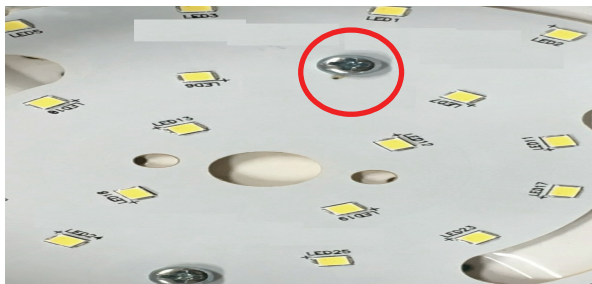
Fig. 3. Withstand voltage test unsuitable sample.
