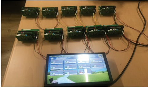
Fig. 11. Communication test of outlet & G/W.
