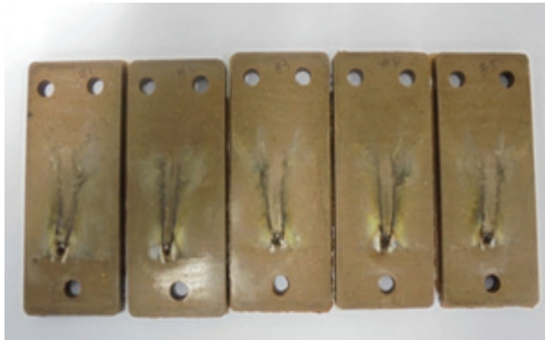
Fig. 2. Vermiculite (10%) tracking test result.
