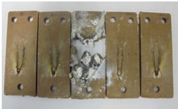
Fig. 3. Vermiculite (15%) tracking test result.
