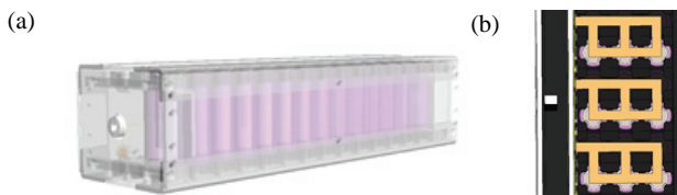
Fig. 1. Battery module design. (a) Module modeling and (b) spot welding point.
