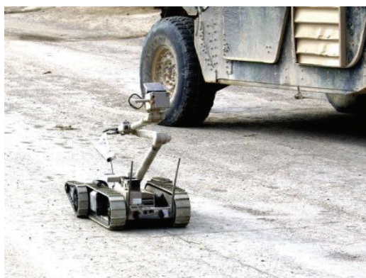
Fig. 1. A robot system for detection and removal of explosive devices.
