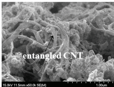
Fig. 7. SEM view of the CNT paste after the surface treatment by Ar ion beam with 100 eV acceleration energy for 15 min.
