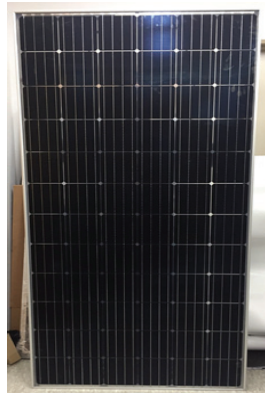
Fig. 4. 6×10 Bifacial PV module fabricated.
