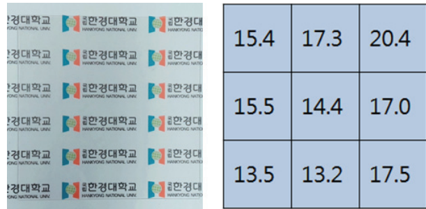
Fig. 6. Snapshot and 9 points sheet resistance of the film fabricated by MOCVD/AgNW method.
