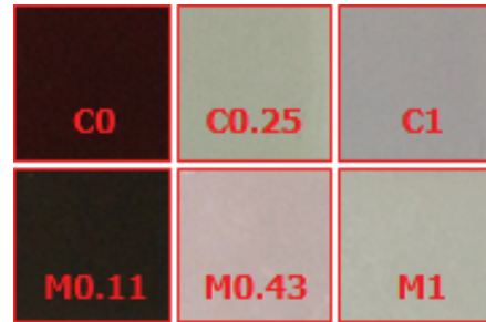
Fig. 1. Images of physical appearance of \text{TeO}_x thin films fabricated by using \text{TeO}_2 and Te targets.
