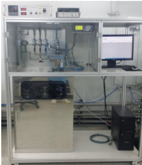
Fig. 3. Measurement system for gas sensing characteristics.
