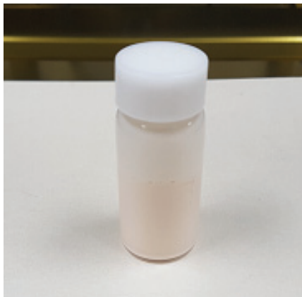
Fig. 3. Wavelength conversion phosphor paste.
