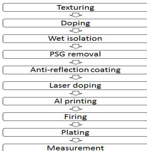
Fig. 1. Fabrication procedure for solar cell.
