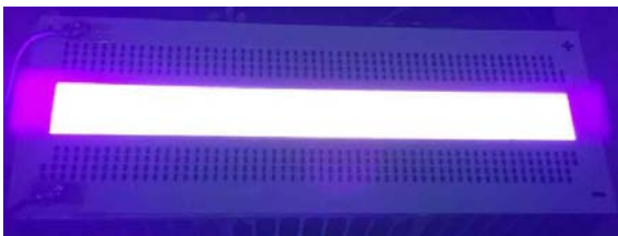
Fig. 5. Fabricated 350 \times 90 \text{ mm}^2 size light source module in operation.
