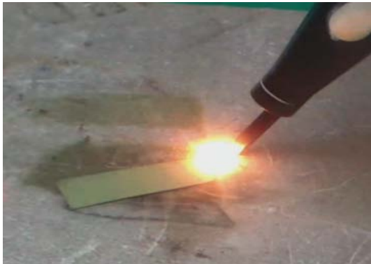
Fig. 10. Ignition tests of Zr/BaCrO 4 heat papers.
