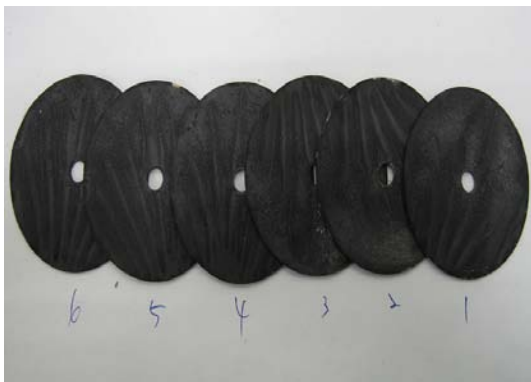
Fig. 11. Heat pellet ignition tests by Zr/BaCrO 4 heat papers (Zr 20 wt.%).
