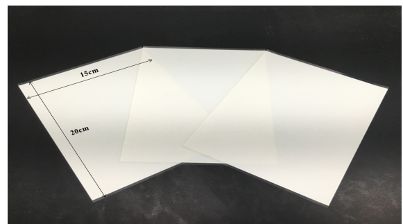
Fig. 2. Piezoelectric green sheets fabricated by a tape casting process.
