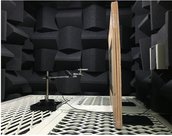
Fig. 5. Image of the semi-anechoic chamber for sound quality evaluation in this study.
