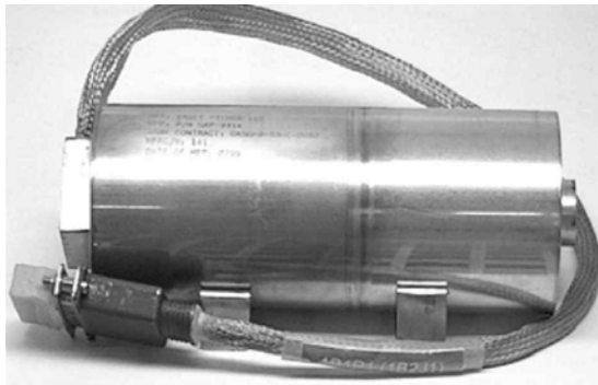
Fig. 1. High-power 1 kW Li/oxychloride reserve battery [1].
