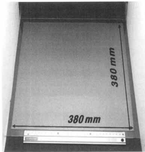
Fig. 12. Photograph of large area deposited PZT thin film on glass substrate. Film thickness is 5.5 \mu\text{m} .
