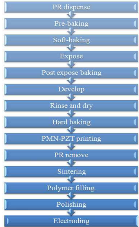
Fig. 1. The picture of Manufacturing process of the micro pillar structure.
