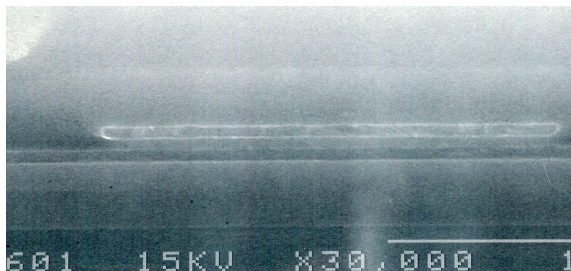
Fig. 1. The SEM image fabricated n channel poly-Si TFTs gate region (X30,000).
