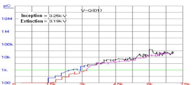
Fig. 11. V-Q result for degraded cable at the rate of 100% (cable length of 30 cm).
