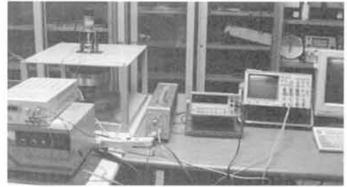
Fig. 6. Experiment apparatus for measurement of magnetization curve.
