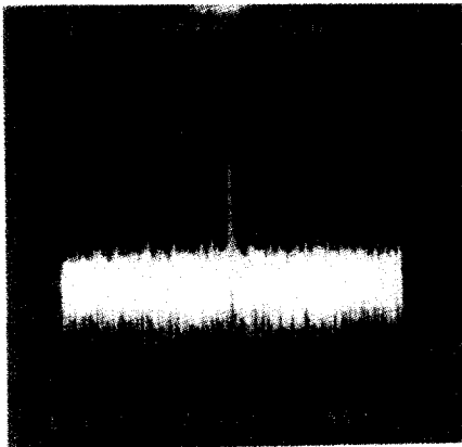
(a) Down-converted IF(=116 MHz).
